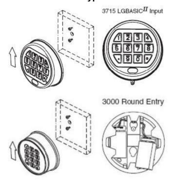
Slide the housing up, carefully pull away from mounting surface to expose battery compartment. **CAUTION! Hold onto battery terminal to avoid pulling wires out of housing.**
