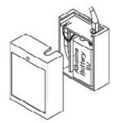
If the battery is completely depleted, place a 9v battery on the 'snake eyes' on the outside of the keypad, hold the battery there for the entire time while you enter the code and open the lock. There is a battery box located on the inside of the safe/cabinet which houses the battery. Please refer to your cabinet manufacturer for the exact location. The lid of the battery box can be lifted and the new battery is placed
